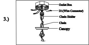
Step. 3: Wire fixture to wires in outlet box. Copper wire is for Ground. Pull canopy through screw ring up chain to ceiling and tighten securely
