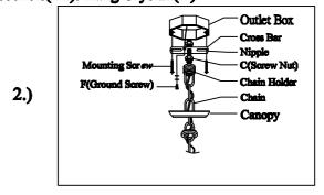
Step.2: Attach cross bar to mounting bracket.
