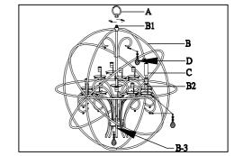
Step.1: Install top loop(A) to center stem(B1) and attach desired amount of chain to loop to achieve desired mounting height. Thread wire through every 3rd loop of chain. Place Candle Covers(C) over sockets(B2). Hang Crystal (D)
