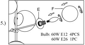
Step 5: Install 60W watts candelabra bulb and E26 medium base bulb (Only for bottom socket). Then install glass (F) into cup (E).
