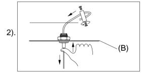
Step.2: Press the wire restraint to adjust the desired length of cable and secure the cables with lock and screws.
