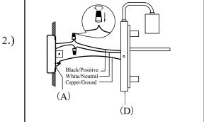
Step2: Wire fixture to wires in outlet box. Copper wire is for Ground.
