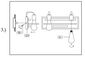
Step3: Install lamp body to back plate using two screws on side. Install bulb into socket.
