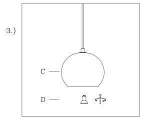
Step. 3: Carefully remove body from fixture. Adjust cable length to desired mounting height, and tighten strain relief screws to secure. Install body (C) to bracket (A) and tighten screws on the sides of the canopy (B) to secure. Screw in GU10(D).
