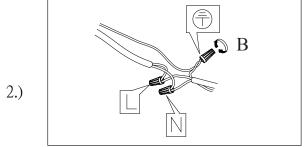
Step.2: Wire fixture to wires in outlet box. Green/Copper wire is for Ground.
