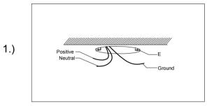
Step 1. Bring positive, neutral, and ground supply conductors (120V, 60Hz) to the room side from junction box(E).
