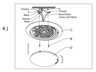
Step 4. Line the acrylic shade up with the bumps on the pan .Twist the acrylic shade until it is secure.
