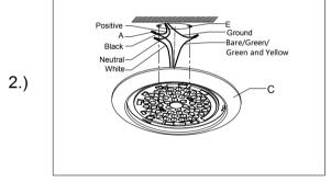
Step 2. Connect black fixture wire to positive, white fixture wire to neutral, and bare copper wire to ground using wire nuts provided.
