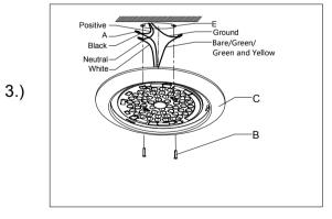
Step 3. Mount the mounting bracket (C) to the junction box(E), using mounting screws(B).
