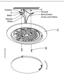
**Mounting:** These fixtures mount directly to most standard metallic & non-metallic electrical boxes with 2-3/4" to 3-1/2" hole spacingthat are at least 1-1/2" deep. This includes 3-1/2" & 4" octagon boxes, round mud-rings for octagon and square boxes, and 3" & 4"non-metallic round boxes. Products are suitable for mounting on ceilings or walls, and are acceptable for use within closet storage spaces when installed per NEC requirements.
