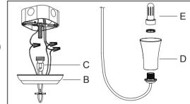
Step3:Install top loop to center stem and attach appropriate amount of chain to loop to achieve desired mounting height. Thread wire through every 3rd loop of chain.Remove ring from loop and slide down chain. Place canopy onto chain and let slide to top of fixture. Install nipple and cross bar into top of chain loop. Wire fixture to wires in outlet box. Copper wire is for Ground. Pull canopy through screw ring up chain to ceiling and tighten securely.
